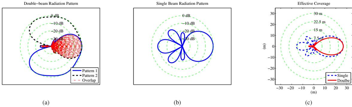
Fig. 4. Radiation patterns and predicted effective coverage of single beamforming pattern and double-beam switching.
