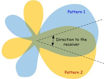
Fig. 2. Illustration of a pattern pair for beam switching.
