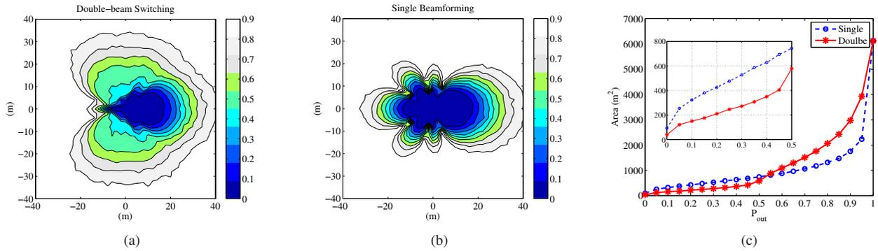
Fig. 8. Outage Probability under single pattern beamforming and double-beam switching in shadow fading channel.
