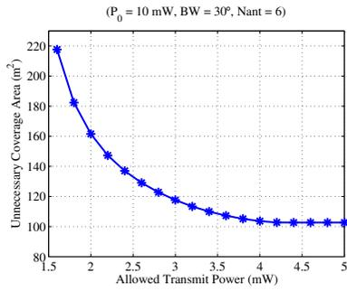
Fig. 6. Minimum unnecessary coverage area v.s. transmit power limit.
