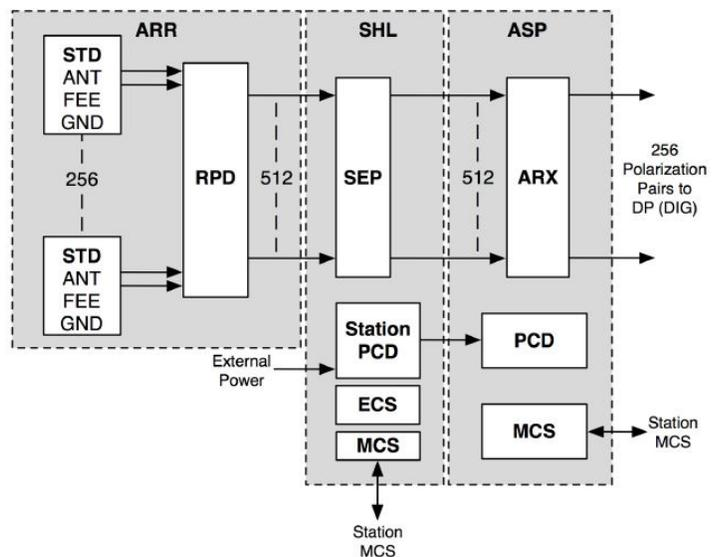
**Figure 10: Architectural schematic of LWA from antennas through analog signal processing.**
