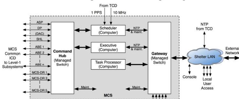
Figure 13: Architecture of LWA monitor and control system.
