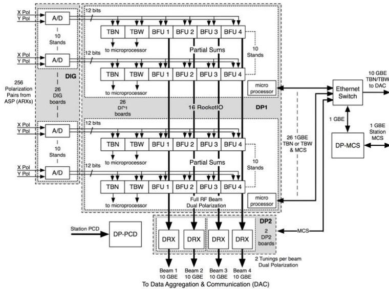
**Figure 11: Architectural schematic of LWA electronics, from digitization through digital processing.**
