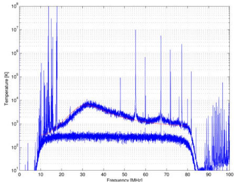
**Figure 14:** *Top curve:* Spectrum acquired in the field using an LWA prototype active antenna (similar to the one shown in Figure 3), with the FEE, ARX and A/D described in the text, with 1 s integration. Also shown overlaying the top curve is the result (red line) predicted from a sky model. *Bottom curve:* Same measurement performed with a 100-ohm (matched) load replacing the dipole arms.
