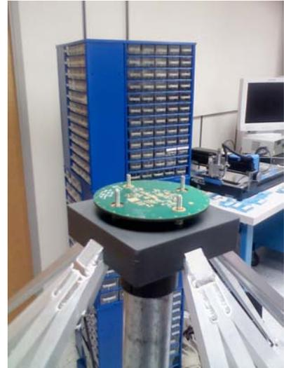
**Figure 9: (left) Schematic view of a single stand; (middle) Photo of stand in lab, showing front end electronics (FEE) box; (right) View of FEE board.**
