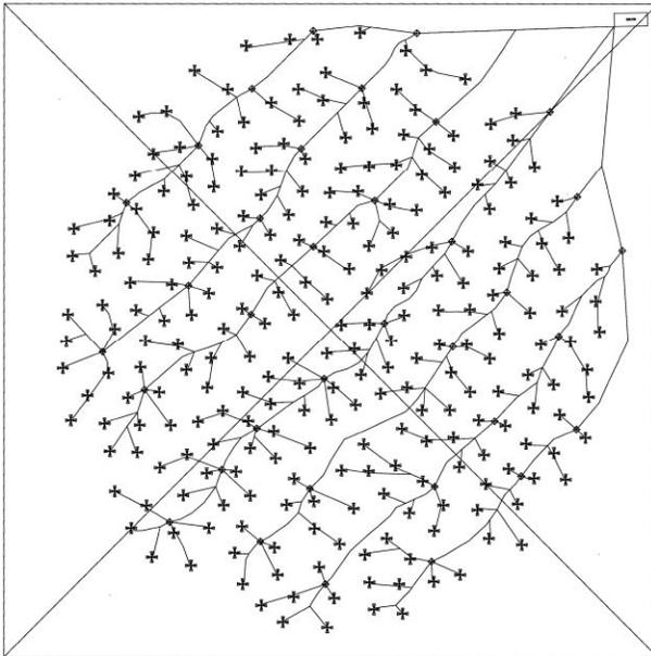
**Figure 8: Stand layout within LWA-1, showing cabling and (upper right) electronics shelter.**
