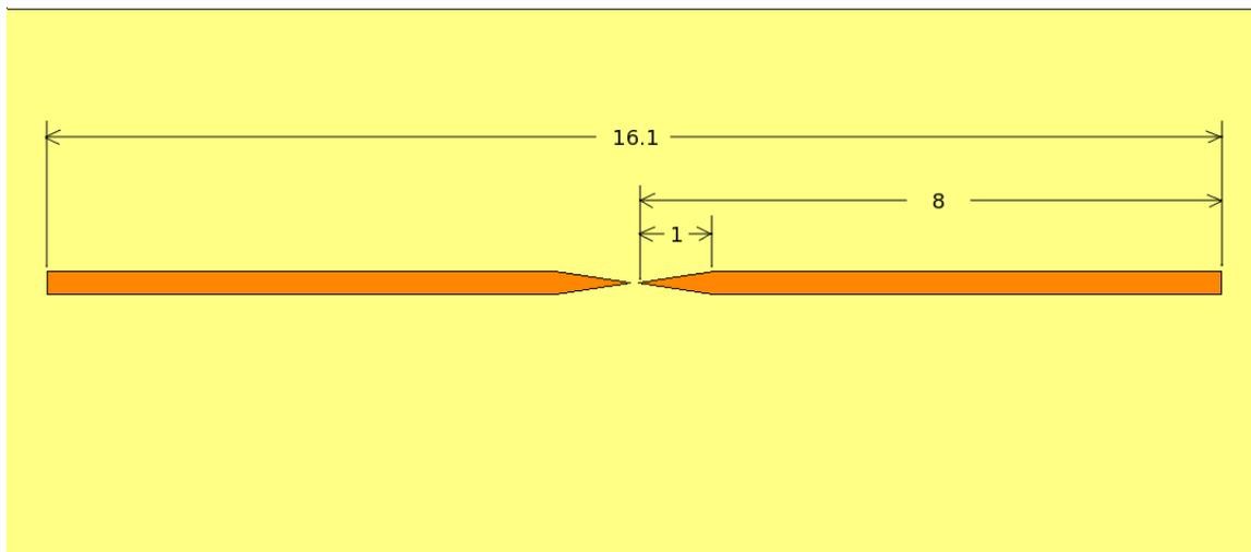
Figure 1: Antenna dimensions in meters.
