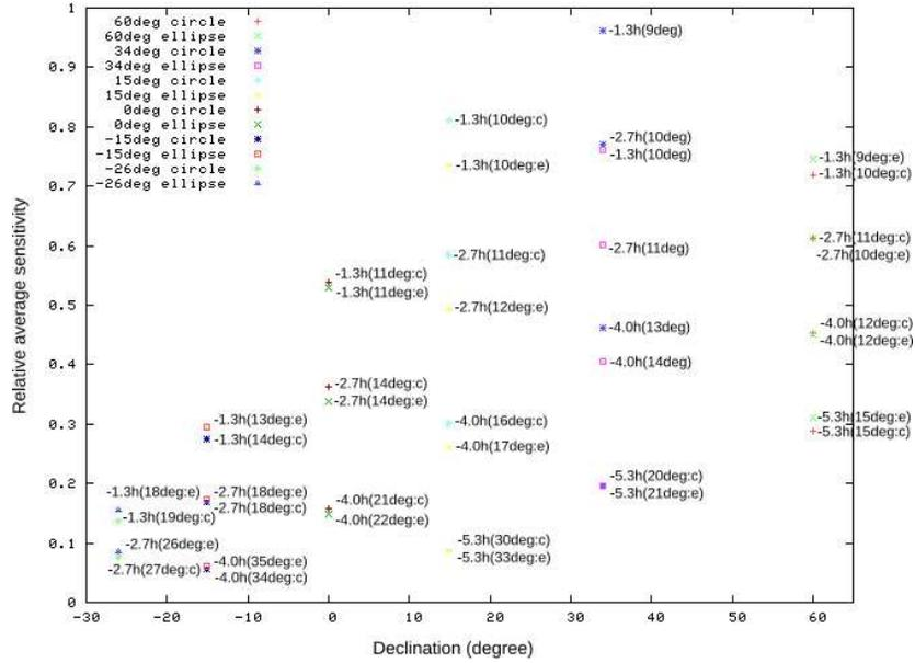
Figure 11: Summary of the averaged direction sensitivities and HPBW at the observing frequency of 20MHz. Each number, such as -1.3h, -2.7h, shows a tracking start hour angle. For example, a -1.3h means tracking from -1.3h to 0h.
