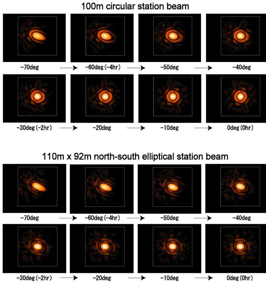
Figure 1: Above shows variations of a circular (top) and elliptical (bottom) station phased beam at 20MHz when tracking in the HA range from  $-70^\circ$  to  $0^\circ$  ( $-4.7^h$  to  $0^h$ ) at  $\delta_{dec} = 34^\circ$ . The simulation was performed using the station located at the latitude of  $\sim 34^\circ$ .
