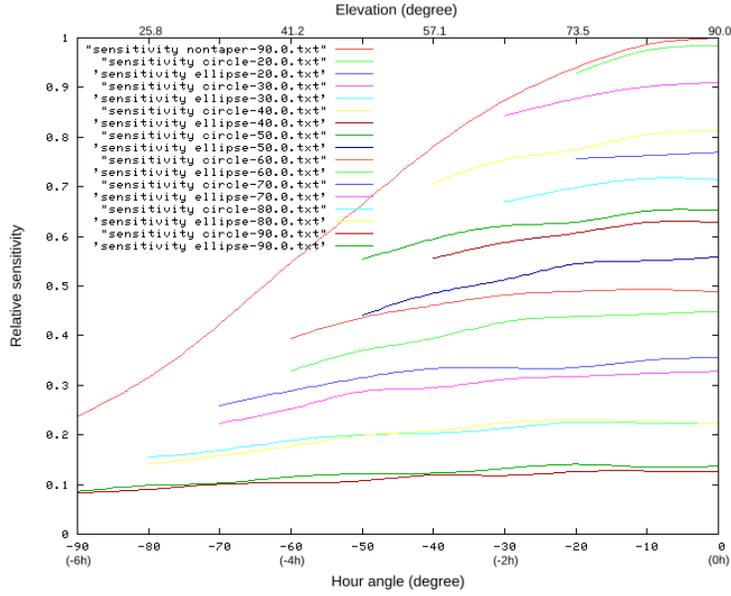
Figure 5: A Comparison of the sensitivities at 20MHz at the declination of  $34^\circ$  with the beams of a 100m circular tapered station, 110m  $\times$  92m elliptical tapered station and no tapered station (the red long steep line).
