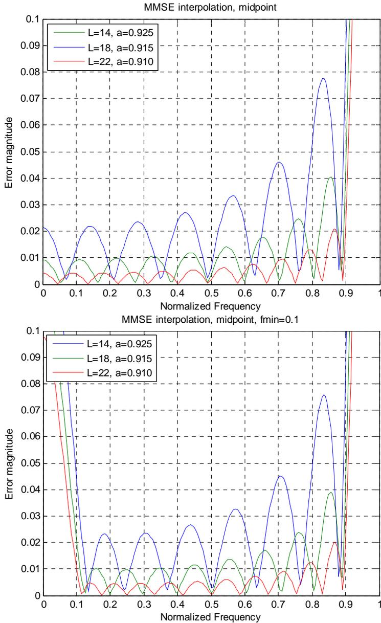
**Figure 1:** Interpolation error magnitude vs. frequency for MMSE error interpolation filters of length 14, 18, and 22 taps. Top: mean square error minimized over normalized frequencies 0 to approximately 0.9. Bottom: error minimized over normalized frequencies 0.1 to approximately 0.9. Interpolation is to the midpoint between samples; the error is smaller for all other fractional-sample interpolation
