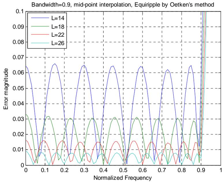
**Figure 2:** Error magnitude vs. frequency for minimax filters of length 14, 18, 22, 26 taps, based on code from [10]. Maximum error is minimized over normalized frequencies 0 to 0.9.
