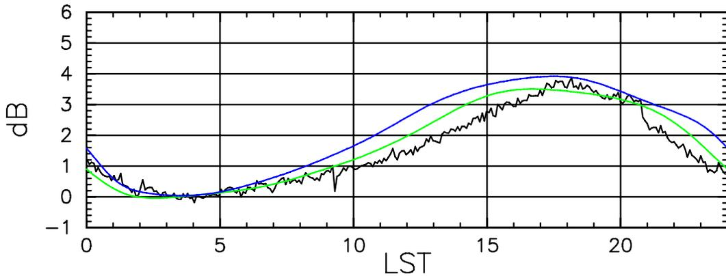
Large Blade Dipole, A Dipole (N-S) 75.23 MHz Offset -34.2 dB
