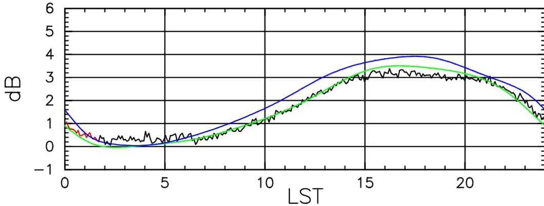
Large Blade Dipole, B Dipole (E-W) 75.23 MHz Offset -33.9 dB
