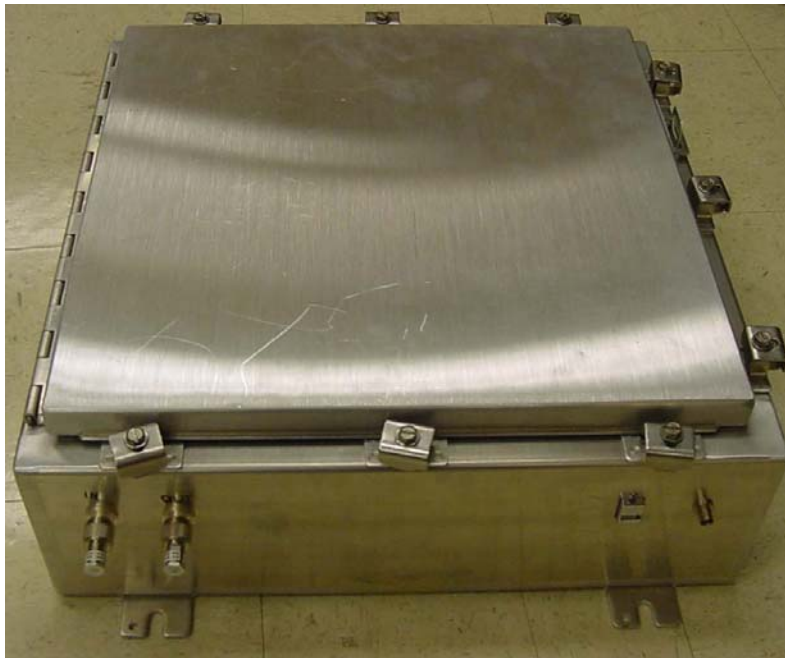
Fig. 7 Pictures of the NEMA enclosure used for field testing of the LWDA receive chain with top lid open (upper) and closed (lower). Note that the steel wool used for RF gasketing in preliminary emissions measurements is not shown.
