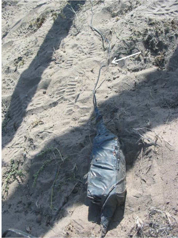
Fig. 9. The 8V power supply for the Hicks balun. The duct tape that had been wrapped in was chewed in several places, and the thin wire connecting the power supply to the balun had been chewed through completely (indicated by white arrow).
