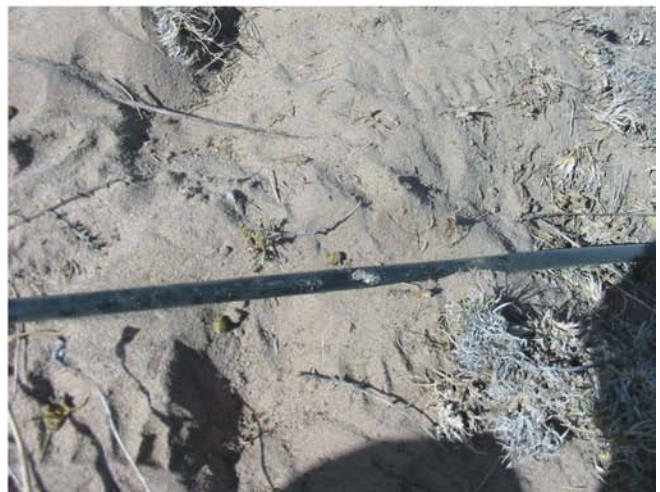
Fig. 10. The power cable (right) and coaxial cable (left) exhibited bite marks along their full lengths. Damage was extensive enough for the copper wiring inside to be exposed in some places.
