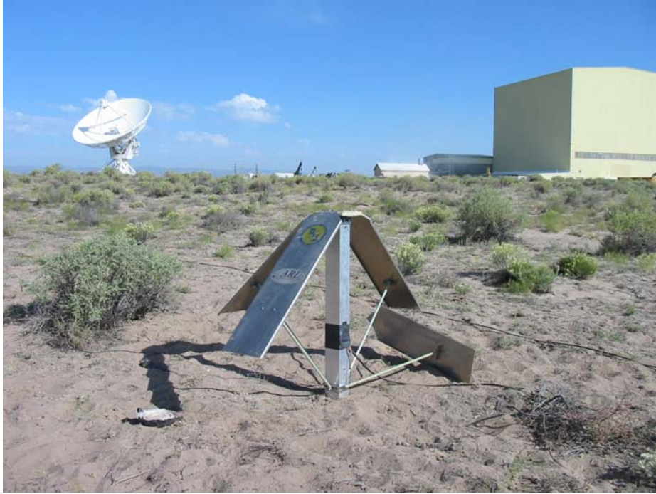
Fig. 7. The damaged blade antenna. One blade was detached from the mast.
