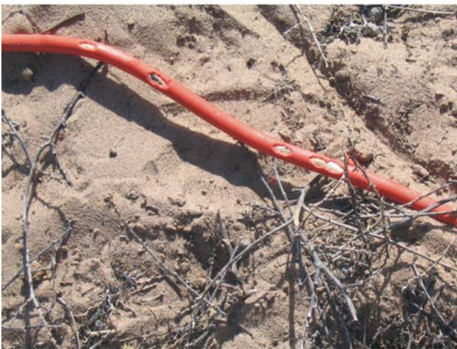
Fig. 10. The power cable (right) and coaxial cable (left) exhibited bite marks along their full lengths. Damage was extensive enough for the copper wiring inside to be exposed in some places.
