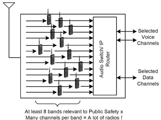
Fig. 1: Conceptual view of the user-based interoperability radio.
