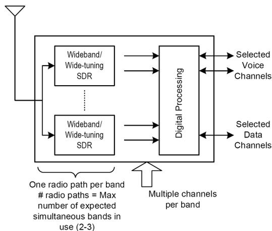
Fig. 2: Functional view of the proposed radio (shows receive side only; transmit side is similar to this).
