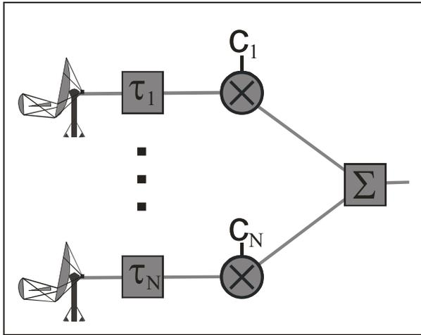
Figure 1: A schematic diagram of the ATA single-tap beamformer. The RF signal from each antenna is delayed and multiplied by a single complex coefficient before summed to give a single-pixel beam.
