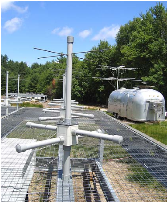
Figure 4: Close up view of the Deuterium Array dipoles showing the directors that have been added to control the horizon response. The trailer in the background has the 12 Yagis of the RFI monitor mounted on it as well as one set of active antennas pointed at zenith.
