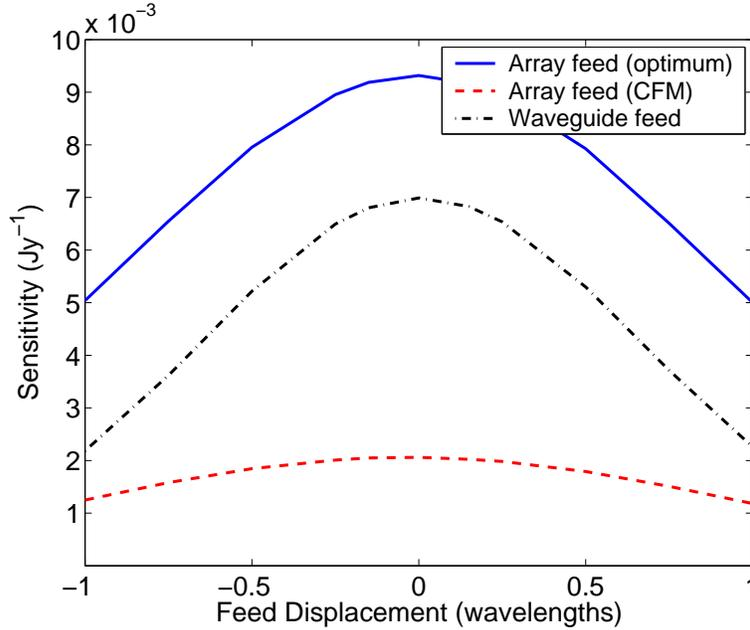
Figure 1: Sensitivity vs. feed offset distance along the paraboloid axis for a seven element dipole hex array (no interferer case).
