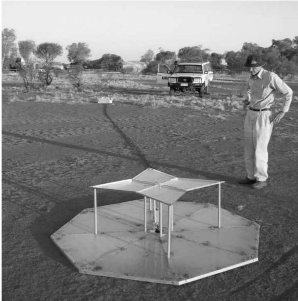
Figure 1: The EDGES fourpoint antenna (from [1]).
