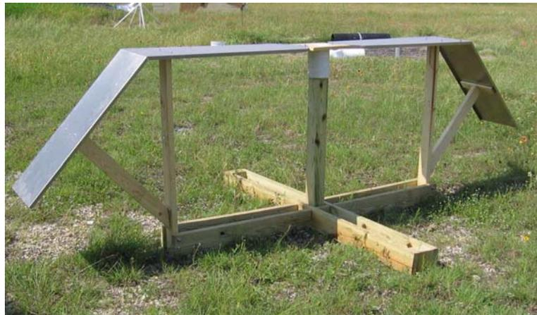
Figure 2. Antennas designs used for drift scan study: big blade (above) and GA-generated design (below). The overall length and height of the big blade is 2.6 m and 1.5 m, respectively. The overall length and height of the GA design is 3.7 m and 1.2 m, respectively.
