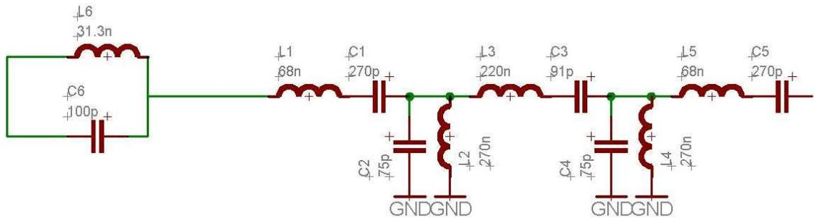
Figure 2: Revised Filter Design .
