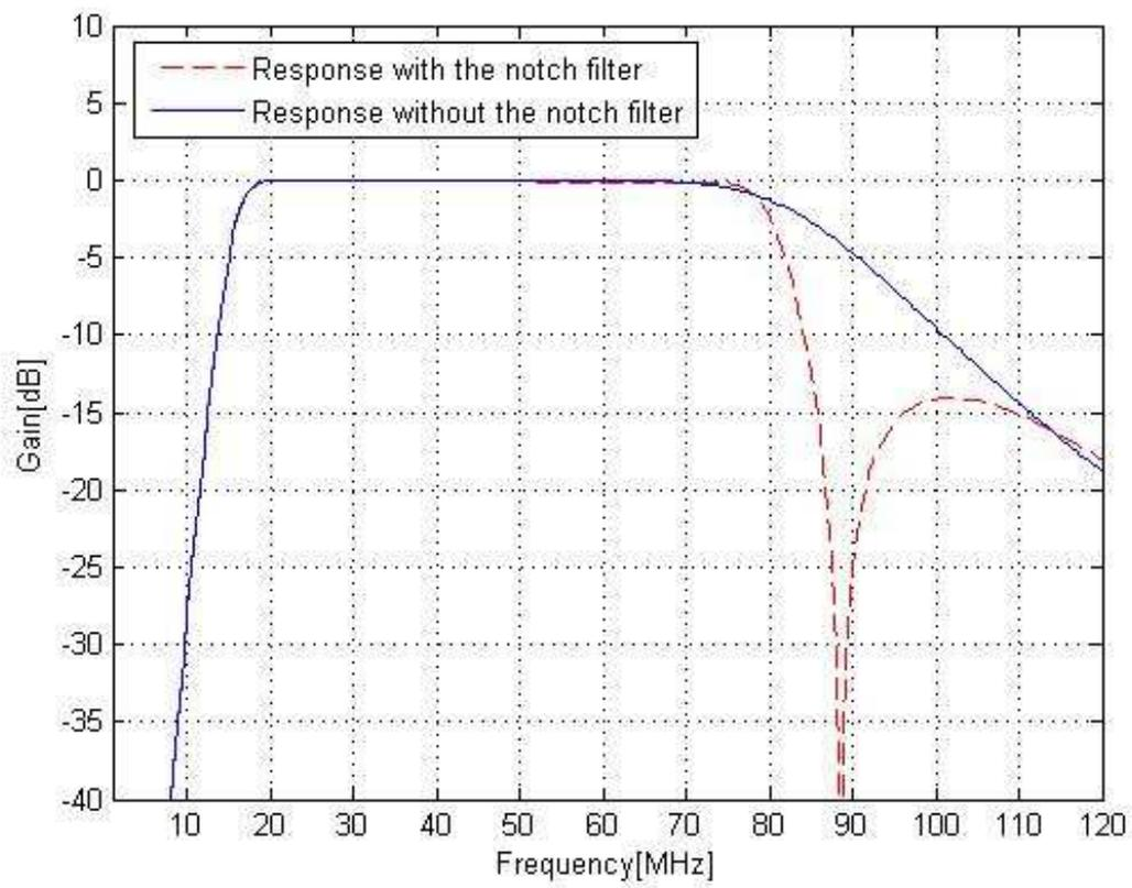
Figure 3: Illustrating frequency responses with and without the notch filter.
