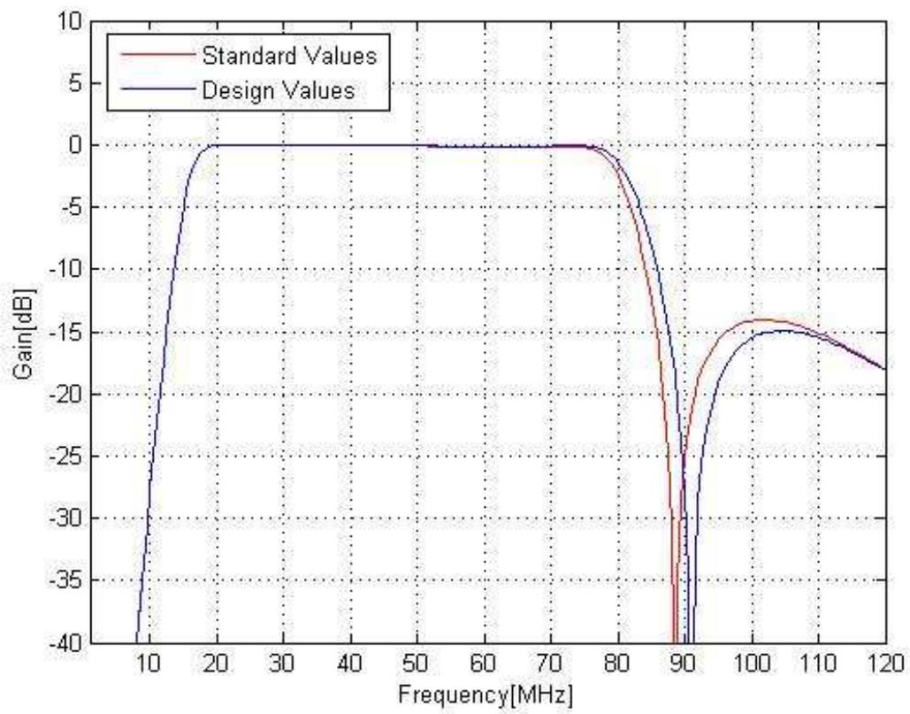
Figure 4: Comparison between responses with standard and design values.
