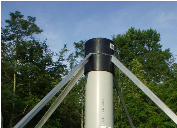
Fig. 2. The ETA antenna stand under test, showing dipole arms and feed region in greater detail.
