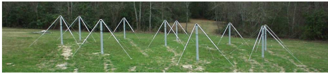
Fig. 1. The 10-element core array of ETA. The antenna under test is in the center. The remaining 9 antenna stands form a circle of radius 8 m.
