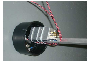
Fig. 4. Mast end cap removed to show mounting of preamplifiers and connection to dipoles.
