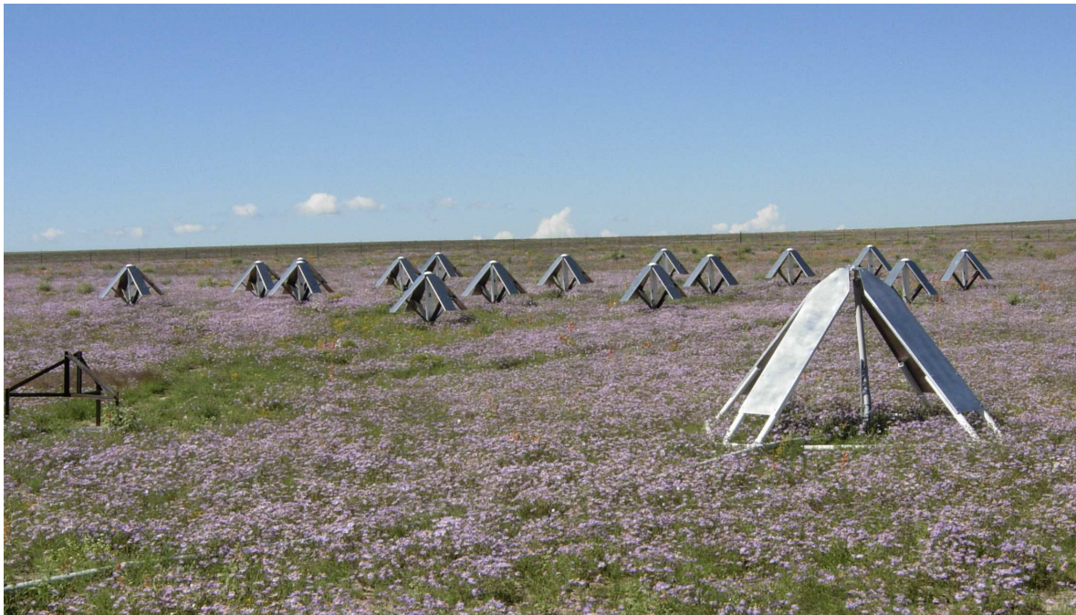
Figure 2.2: A big blade prototype at the LWA site for testing with the 16 LWDA stands in the background taken in August 2006 after a series of heavy rains watered the Plains of San Augustin.
