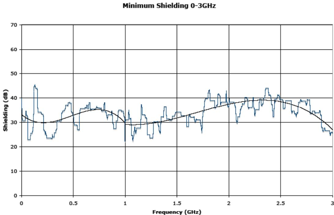
Figure 1. Minimum shielding factor of the LWDA shelter, the blue line is the data and the black solid line is a 3<sup>rd</sup> order polynomial fitted to the data.
