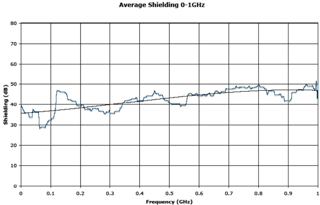
Figure 2. Average shielding factor of the LWDA shelter, the blue line is the data and the black solid line is a 3<sup>rd</sup> order polynomial fitted to the data.
