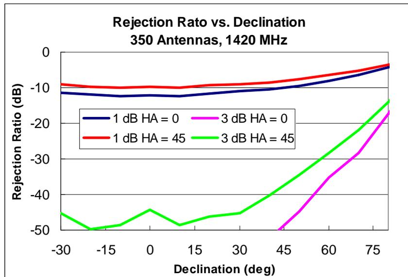
Figure 6: Rejection ratio as a function of declination. Ratios are shown for two discrimination thresholds (1 dB and 3 dB) and for two hour angles ( $0^\circ$  = transit, and  $45^\circ$ ). The rejection ratio gets noisy at very low levels due to the finite number of sidelobe samples in the calculation.
