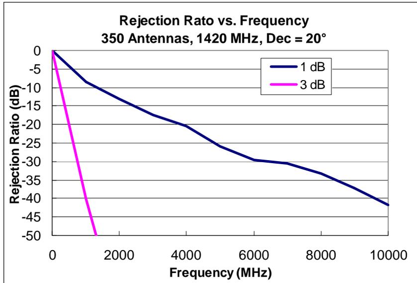
Figure 7: Rejection ratio as a function of frequency. As the frequency increases, the sidelobes become smaller and the rejection ratio improves.
