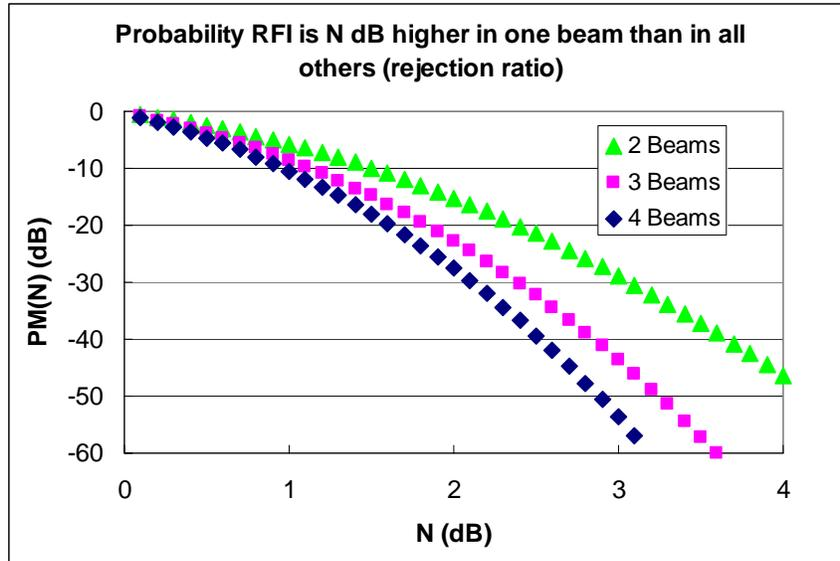
Figure 5: Similar to fig. 3, the probability that RFI will appear at least N dB higher in one beam than in all others, but for a 5 minute track. The blue curve is most comparable to fig. 3 and assumes 4 beams are used. The magenta and green curves show the same calculation for 2 and 3 beams, respectively.
