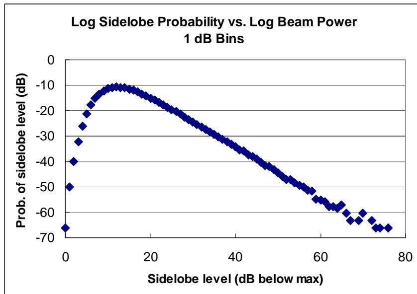
Figure 2: Numerical estimate of  $P(s)$  in a snapshot observation. This is the probability that a randomly chosen sidelobe will have a level within 0.5 dB of a specified level, as a function of sidelobe level. Levels are measured from the maximum sidelobe level observed (excluding the beam maximum).
