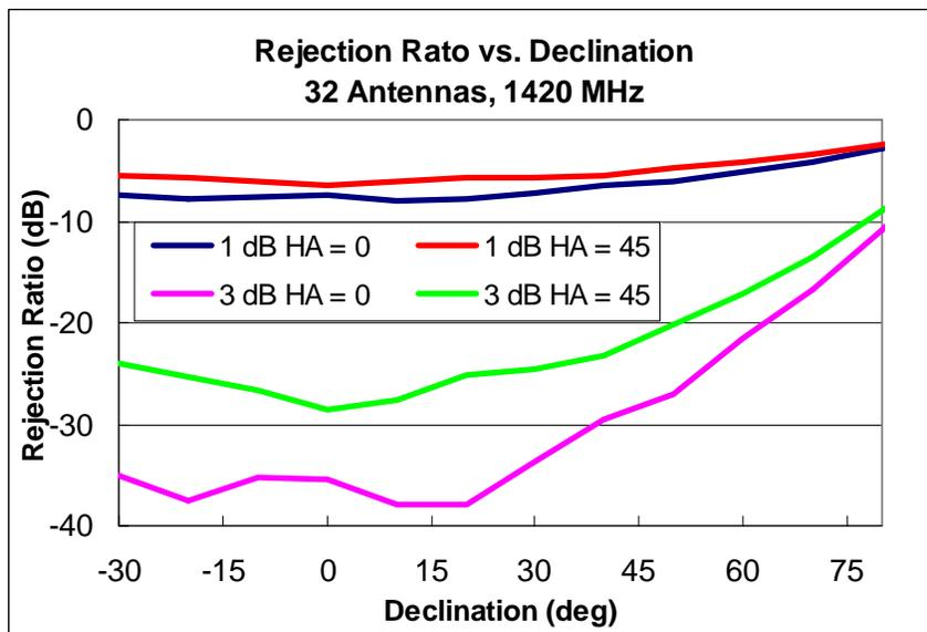
Figure 8: Rejection ratio as a function of declination for the ATA-32 configuration. Because there are fewer antennas and the spatial extents of the array are smaller than ATA-350, the rejection ratio is lower than for ATA-350, but still useful.
