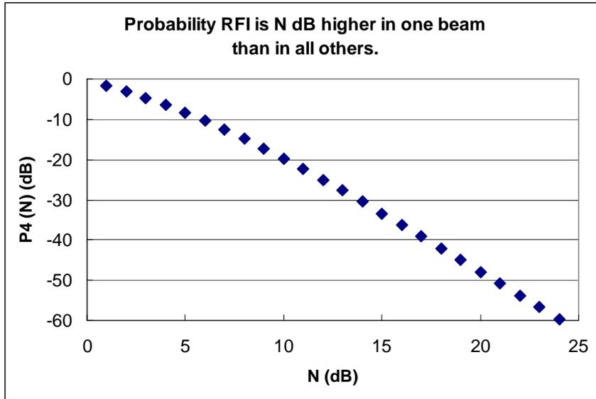
Figure 3: In a snapshot observation with four randomly placed observation beams, this graph shows the probability that one beam will exhibit RFI at least N dB higher than the same RFI in the other three beams. For example, the RFI will appear in one beam at least 10 dB higher than in all other beams about 1% of the time ( $P \sim -20$  dB).
