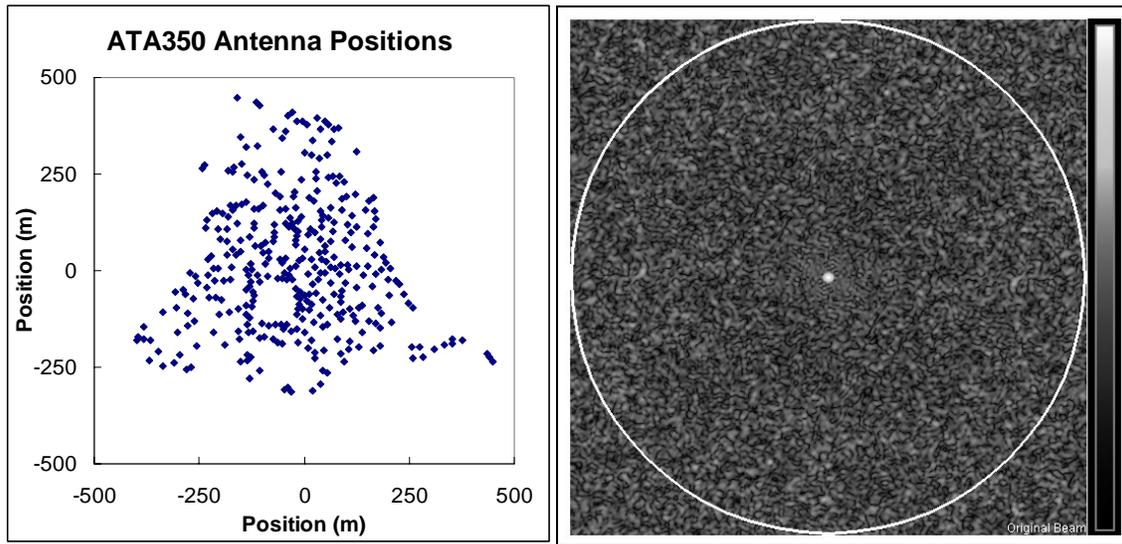
Figure 1: Left: Proposed layout of ATA-350 antennas. Right: Portion of the synthetic beam pattern of ATA-350 including the synthetic beam peak. The color bar identifies sidelobe power as measured from the maximum value in the image where white = 0 dB and black = -50 dB. The white circle shows the ATA primary beam FWHM.
