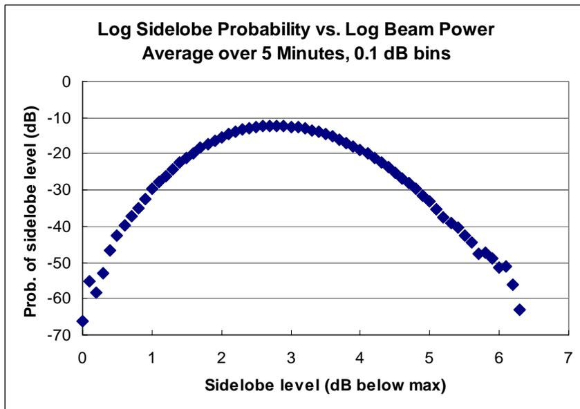
Figure 4: Similar to fig. 2, the probability that a randomly chosen sidelobe will have a level within 0.05 dB of a specified level, as a function of sidelobe level. This calculation results when the beam power at the RFI position is averaged over a 5 minute time period (source declination  $20^\circ$ ).
