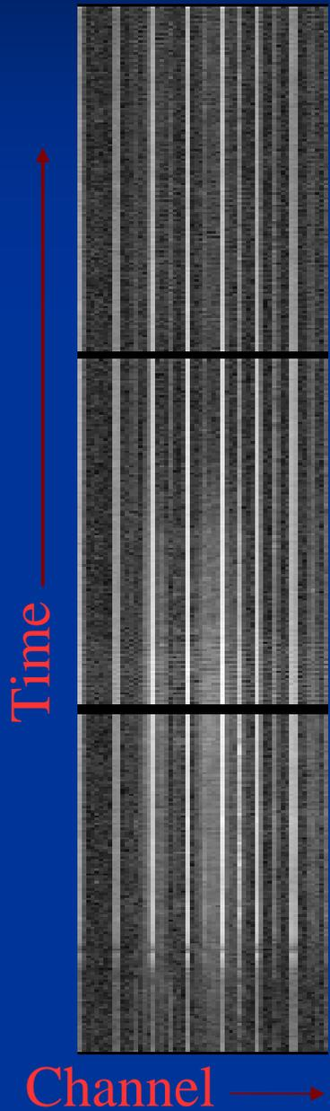
Internally generated rfi “comb” at 100 kHz
